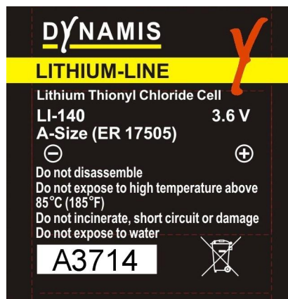
LTC cell marking example
